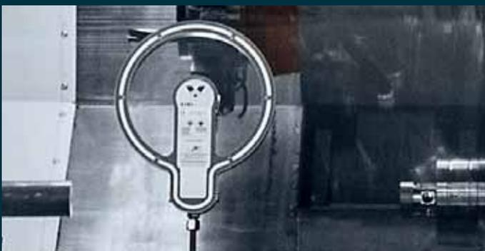
**Spin window.** The optional spin window enables the optimal insight in the working area, also during machining with coolant. Due to its very fast rotating glass plate, the coolant is slung away immediately after impact and the window stays clear.
