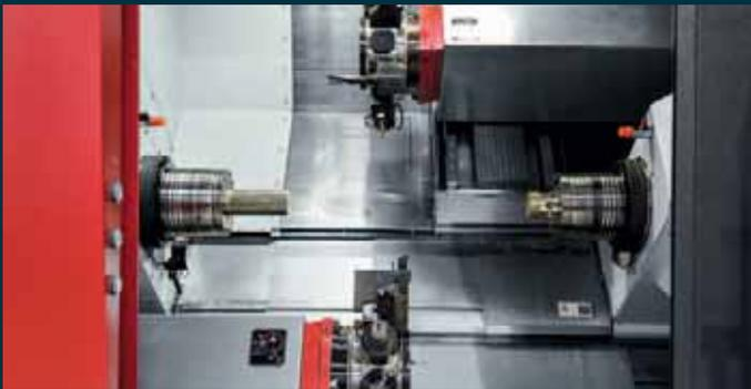
**Tool turret.** Fast 12-station servo turret with very short switching times for standardized VDI30 or VDI40 tools. All stations can hold driven tools for drilling, milling, and tapping. The operator is able to control the indexing speed with the override switch at any time.
