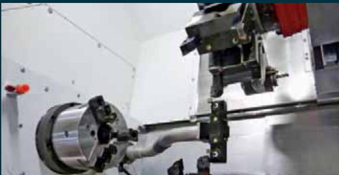
**Tool measuring.** The tool measuring arm equipped with two touch-probes enables fast and precise measuring of tools in the workspace. It is mounted manually in the bracket below the main spindle and returned to a storage tray after use.
