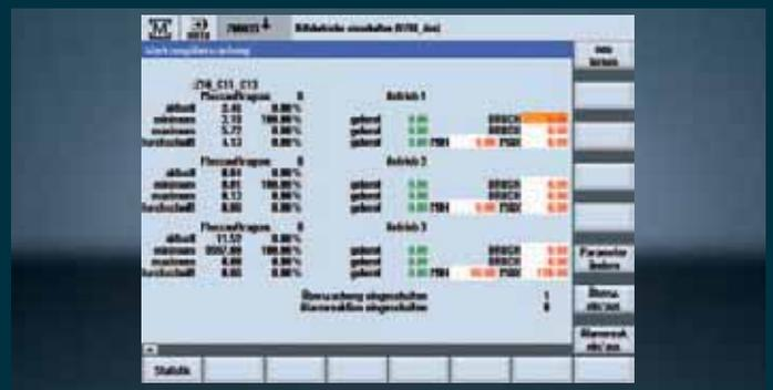
**EMCO tool monitoring system.** The tool status is monitored by evaluating the load on the various axis drive motors. Excessive loads point to tool wear or breakage. Too low a load indicates a tool is missing.
