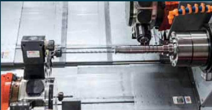
**Deep hole drilling.** For the processing of deep holes, high pressure cooling installations up to 80 / 150 bar with filtration and coolant temperature control are available. Internal coolant supply with stationary but also driven tool heads ensure a save cutting process.
