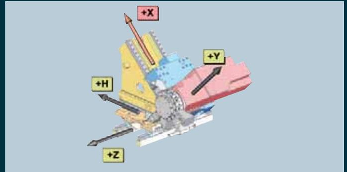
**High-precision Y-axis.** The HYPERTURN's Y-axis is designed to distribute the cutting forces over two guide planes. The result: outstanding rigidity for all turning and milling operations. The  $\pm 50$  mm travel permits off-center milling and drilling.
