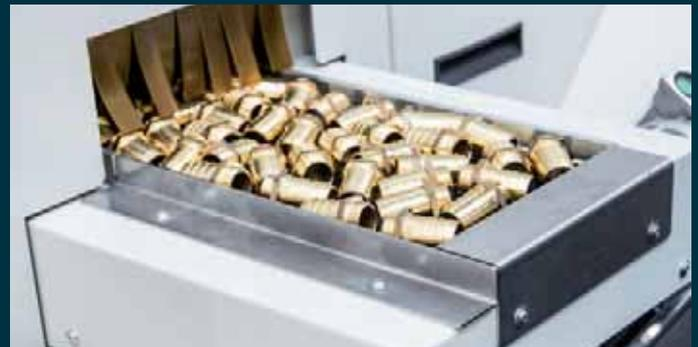
**Prefabricated part conveyor belt.** On the conveyor belt with in the machine casing, arranged lengthwise, with a storage surface of 1400 x 180 mm, the work pieces are put down damage free.
