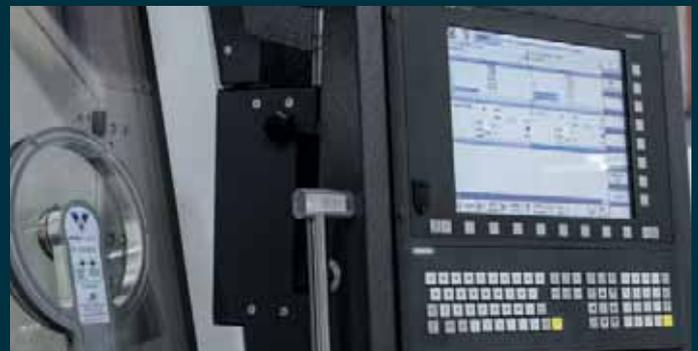
**Control.** The Sinumerik 840 D sl with operate user interface is ergonomically arranged on the right from the working area, can be swiveled 80° and changed in height by 100 mm. A side-to-side movement is standard for the 1300 versions. On the bottom is a 230 Volt socket, which can be used for any electrical device.
