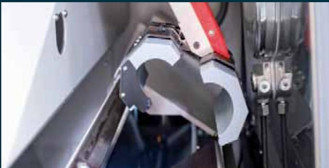
**Parts catcher.** The HYPERTURN 65's electro-pneumatic parts catcher is controlled using M functions. When needed, it traverses to the front of the work area and pivots to the spindle center. The finished part is removed from the clamping device and transferred to the catcher tray. The parts catcher then moves back to its initial position and the part is tipped onto a conveyor belt.
