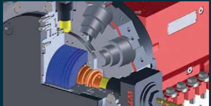
**BMT-turret.** For economical production of complex turned/milled parts with mainly milling share, there is optional the BMT-turret with water cooled direct drive. With max. 12000 rpm, 30 Nm and 10 kW, this turret offers optimal prerequisites for the complete machining.
