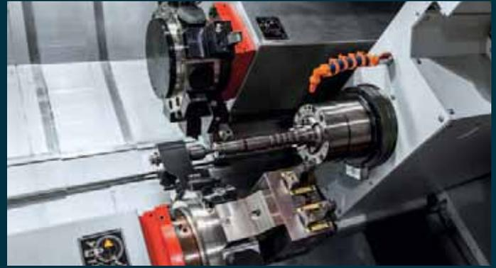
**Live-center / turret-steady-rest.** For complete machining of shaft work on the one hand in the main spindle and on the other hand in the sub-spindle, there are a live center and if needed also a turret steady rest available. So that long, slim workpieces can be manufactured precisely and without chatter marks.
