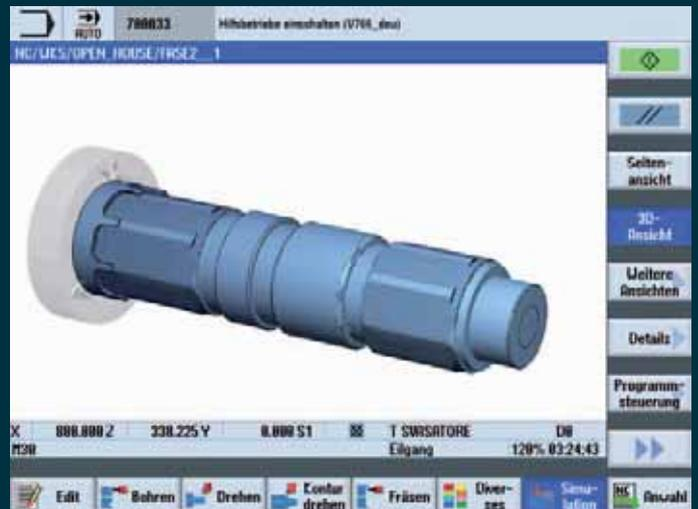
**Machining simulation:** 3D simulation, simultaneous display during the turning and milling - with representation of detail and workpiece cutting. This achieves a significantly higher efficiency in production and all information is available on the machine.
