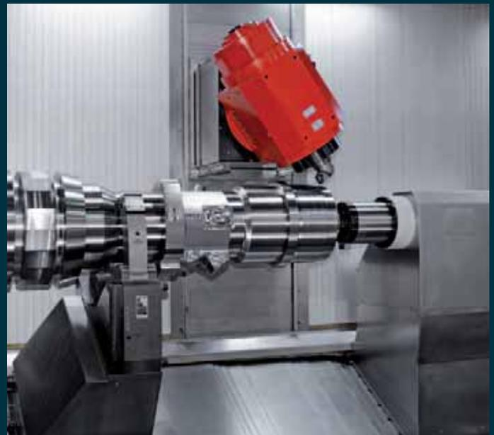
**Tailstock.** The tailstock is 100% programmable using the control. With the high-quality and precisely-dimensioned MK6 quill, all operations can be supported or extended with the counter spindle thanks to the machine modular construction.
