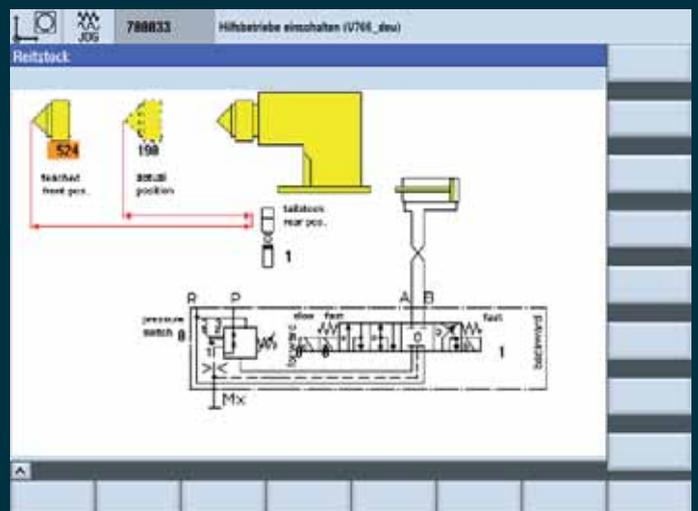
**EMCO Diagnostics:** EMCO Diagnostics for rapid, easy analysis of the whole machine (for example: tailstock hydraulic scheme and quill position monitoring).
