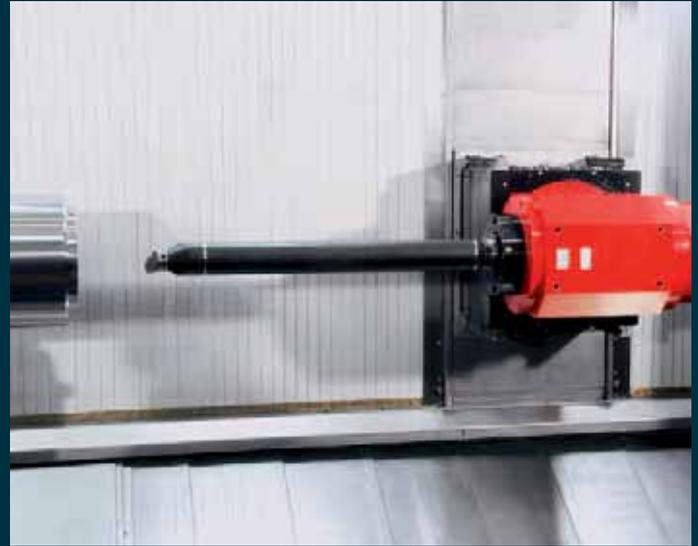
**Turning operations.** External or internal turning operations are possible with the stable spindle in 3° step. Optionally, the vibration-damped boring bar can be equipped up to a length of 1000 mm and with a 3-positions (stations) pick-up magazine.
