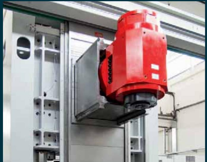
**Moving column.** Is constructed like the EMCO MECOF machines with a „Box-in-Box“ RAM structure. Thus, optimum rigidity and stability are ensured and high accuracy machining is guaranteed. The B-axis is equipped with a torque motor and integrated into the Ram design.
