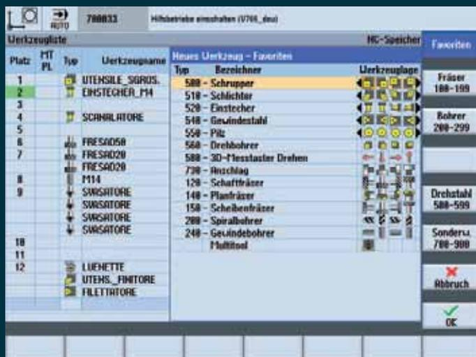
**Tool management:** Simple and open operation through an integrated management tool for all tool types and data.
