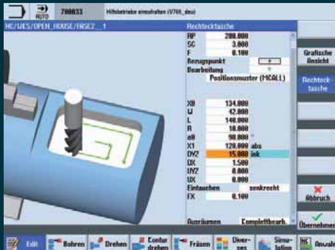
**Shopturn-Shopmill / Machining cycles:** The machine programming can be chosen completely freely from ISO to Shopturn. Complex workpieces require efficient production methods and innovative CNC solutions. The SINUMERIK 840D sl CNC equipment supports multi-technology equipment in the machining of workpieces in one setup and offers innovative functionality for this - even alternating between different technologies.
