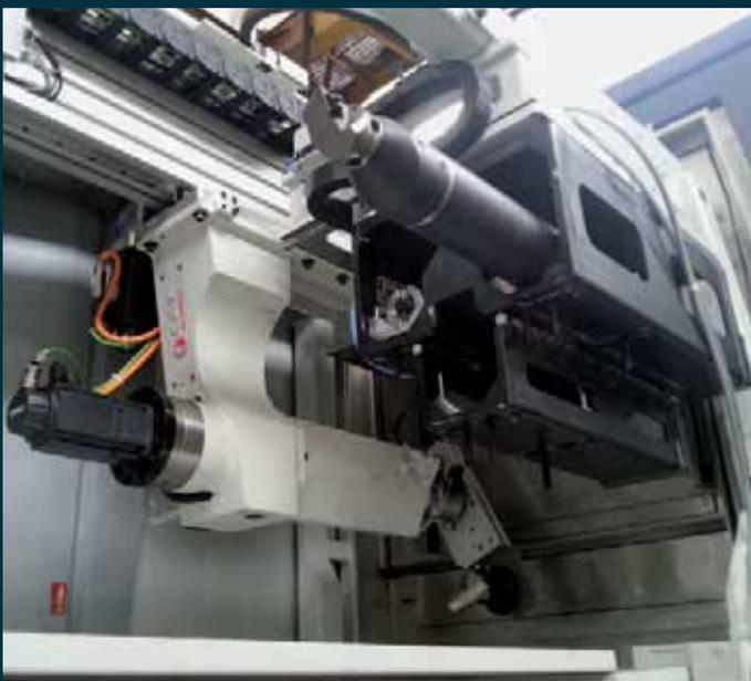
**XL magazine.** Equipped with a 3-positions pick-up magazine, it includes tools up to a length of 1000 mm
