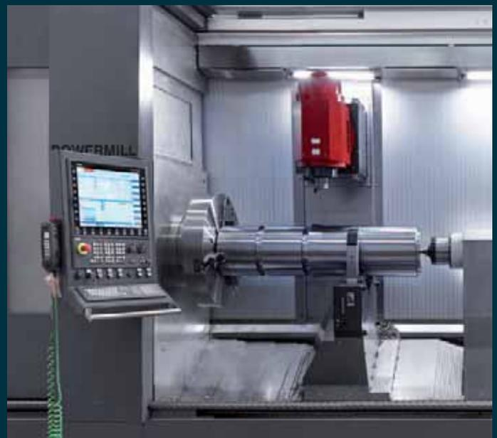
**Machining capabilities.** With this performance profile and workspace dimensions the machine can produce large, complex workpieces with a maximum workpiece weight of 1500 kg in the chuck and up to 6000 kg between the chuck and tailstock.
