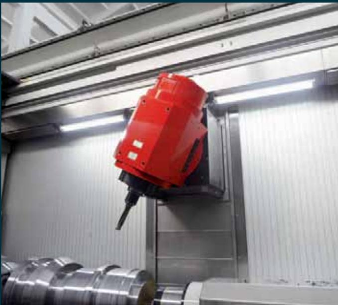
**Milling spindle.** For stable, precise and flexible drilling and milling operations. Up to 80 kW and 630 Nm of torque and 10000 rpm. Sealing air, internal HP coolant with 40 bar and externally with 14 bar and a 1400 liter paper band filter system as standard (80 bar option). The B-axis can be used at any angle or with an indexed B-axis in 2.5° steps.
