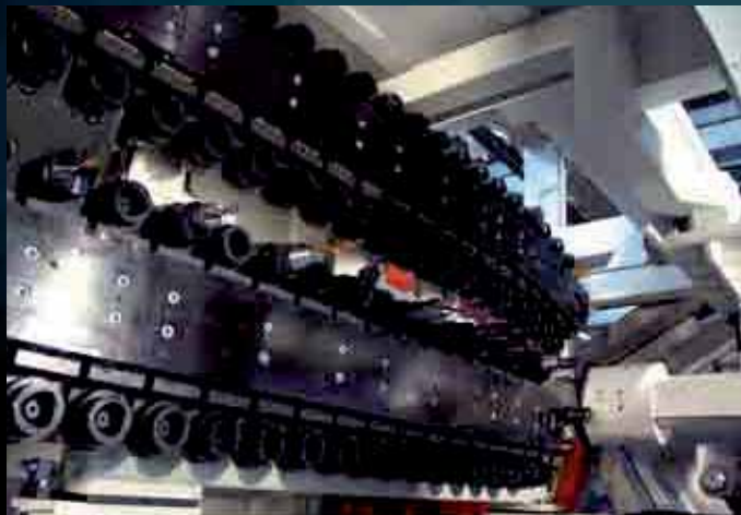
Tool magazine with 80 pockets integrated to machine layout.
