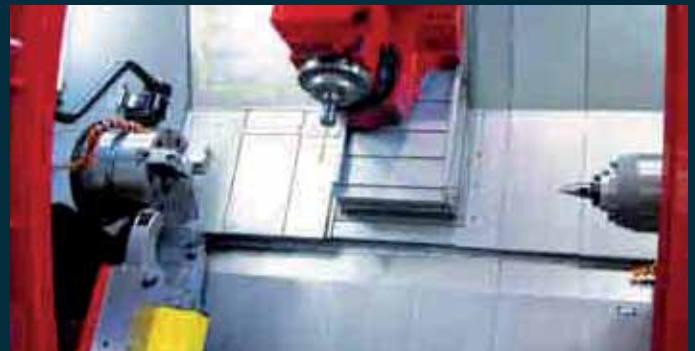
The modular machine concept also enables the use of a tailstock in combination with an NC-controlled steady rest instead of the lower tool turret, depending on the customer's requirements. The steady rest can be hydraulically lowered 250 mm if required.
