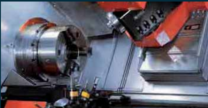
Main spindle view with clamping device \varnothing 315 mm and milling spindle. The lower tool turret is unrestricted when machining workpieces with large diameters.
