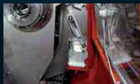
Parts catcher with conveyor: Finished parts are ejected with a coolant fed part ejector into the parts catcher and transferred with a conveyor to a storage area.
