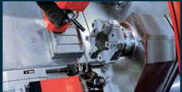
Counter spindle view with 6-position jaw chuck \varnothing 500 mm. The upper turret is replaced by a 21 kW liquid-cooled milling spindle in the B axis version. The B axis travel range is 205°. This is infinitely variable with 0.001° resolution. In addition, the B axis can be clamped in any position with 5° indexing.
