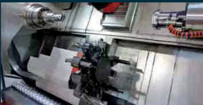
Tool turret: Fast indexing 12 station tool turret for standardized VDI40 or CDI80 (CAPTO) tooling. All stations can be used with driven tools for drilling, milling and tapping operation. The turret indexing movement can be controlled by the operator at any time. Max. turning diameter for lower turret is 650 mm.
