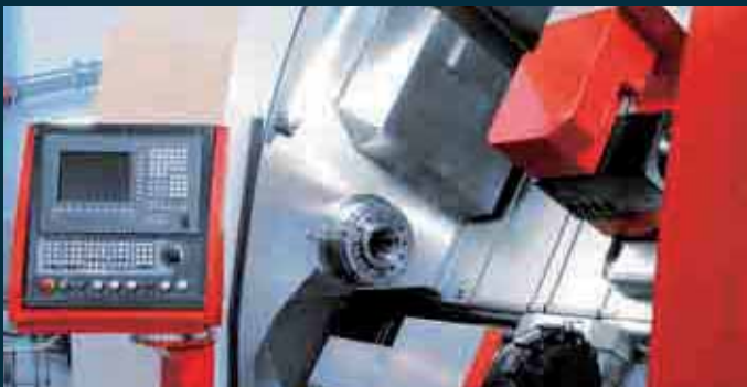
The work area provides the highest level of ergonomics with excellent accessibility to the individual components. Generous amounts of free space ensure optimal chip flow, even when machining complex materials. All guides are covered in stainless steel sheets to prevent damage.
