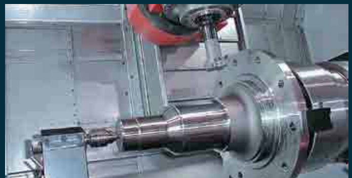
The lower tool turret can be fitted with a live center point and can act as a tailstock for machining large workpieces.
