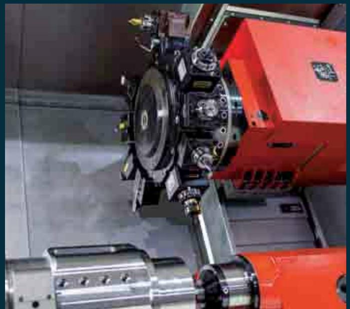
**MT 110 BMT turret.** For cost-effective production of complex turning/milling work pieces, in which milling is predominant, the optional BMT 65P turret with water-cooled direct drive is available. With a maximum of 9600 rpm, 56 Nm and 17.6 kW, this turret offers optimum conditions, stability for complete machining and maximum productivity.
