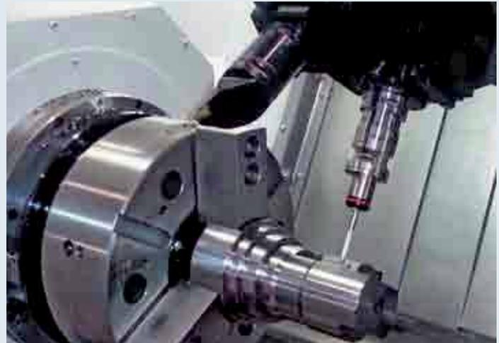
The probe is in the turret with radio transmission for scanning the workpieces and automatic transfer of values used by measuring cycles.
