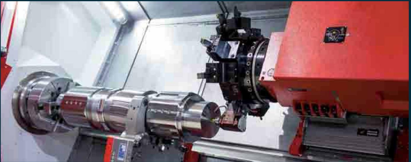
**The Maxturn series** is designed as a modular system with expansion stages from simple turning operations to a turn-mill centre with different application potential: dynamic integrated spindle motor as well as high torque implementations, direct drive turret with BMT or VDI tool holder systems.
