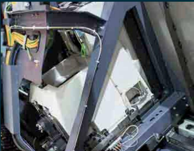
**High-precision Y-axis:** The Maxturn machine concept has been specially developed for placement of the Y-axis at an angle of 90°. Due to large dimensioned, widely spaced and pre-loaded guide ways, the Y-axis offers optimal machining results with maximum stability and short overhangs.
