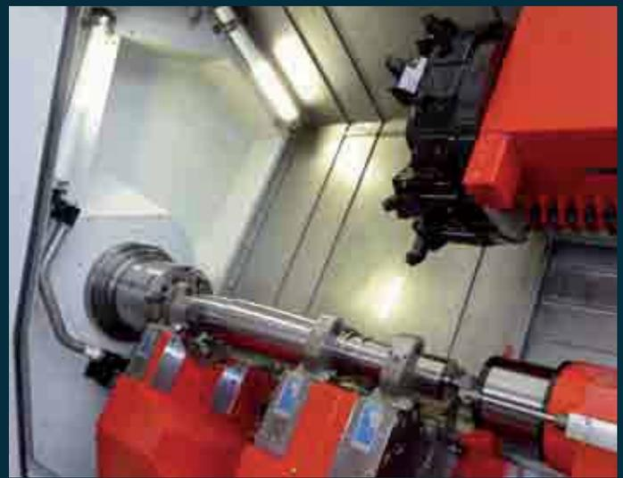
**Steady rests / clamping:** High-precision complete machining is possible with 3 steady rests on two process-driven slides. Optimal productivity with maximum flexibility is provided due to a shaft-chuck with retractable jaws carrier and face driver, as well as tool calibration.
