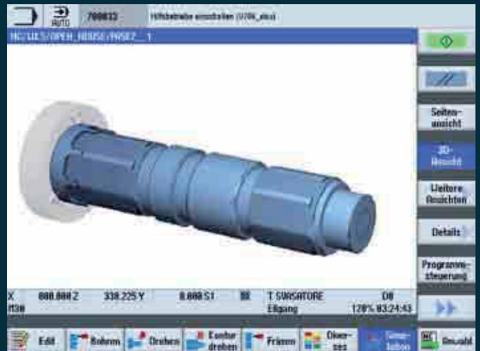
**Processing simulation:** 3D simulation during turning and milling, with detailed representation and workpiece profile
