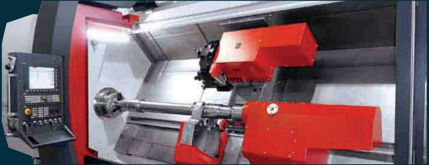
**Maxturn 110 Machine concept:** Best Turn-milling for each machining. Robust and high-precision machine design to the complete to allow creation of long workpieces. The wider door opening, the automatic, stable tailstock with integrated storage and MK6 Pinole (Optional) and a tilting control console for optimal operation and uncompromising handling.
