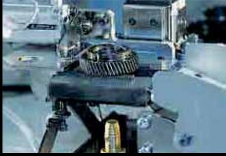
**Measuring device:** Measuring station integrated at the machining table for machining of precision parts with minimum manpower. The tool offsets are adjusted automatically. By means of the gantry loader, each workpiece is placed into the measuring device and measured with the measuring gauge. Good parts are pushed into the parts container, rejected parts are stored separately.
