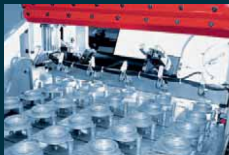
Large storage capacity chain feeding system for loading preformed blanks with the correct orientation.
