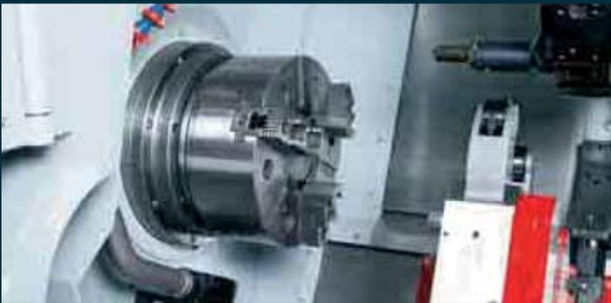
**Main spindle.** Two versions are available. One using a conventional beld-drive for high torque (up to 1040 Nm) and heavy machining and another one using the approved water-cooled motor spindle for higher spindle speeds. This one also offers optimal conditions for complex milling operations.
