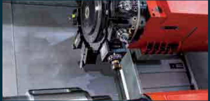
**BMT turret.** For cost-effective production of complex turning/milling work pieces, in which milling is predominant, the optional BMT 55P turret with water-cooled direct drive is available. With a maximum of 12000 rpm, 30 Nm and 10 kW, this turret offers optimum conditions, stability for complete machining and maximum productivity.
