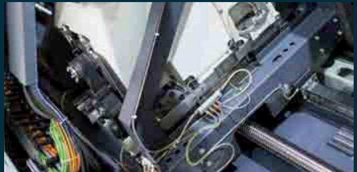
**Y-axis.** The Y-axis forms a highlight in the MAXXTURN series. She is integrated in the machine structure so that maximum stability based on short overhangs and wide distanced roller guides is guaranteed. Thus, complex machining tasks can be done and workpieces can be completely finished in a single setup. A variety of machining cycles in the controller allows easy programming and the use of the additional linear axis.
