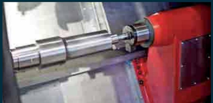
**Tailstock.** The tailstock is mounted on linear roller-type slides and can be positioned via the z-axis-slide. Optionally an additional servo drive using a ball screw can be offered. At the determined position the slide is hydraulically clamped. So that a quill with integrated bearings and MT4 cone can support the workpiece. Therefore the quill can move up to 120 mm.
