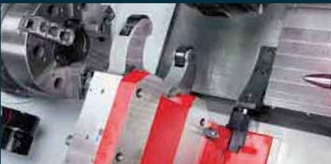
**Steady-rest.** The hydraulic operated self-centering steady-rest has a clamping range of  $\varnothing$  30 – 245 mm. It is mounted on a slide, which can be positioned via the Z-axis-slide or optionally via an additional servo drive using a ball screw. At the determined position the slide is hydraulically clamped. The steady-rest includes chip protection and central oil lubrication.
