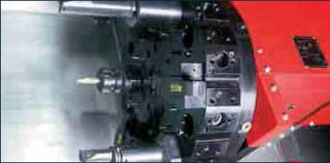
**Tool turret:** 12 + 12 station hybrid tool turret - VDI40 + block-tool, axial turret with single-motor technology. A servo motor powers the driven tools and the swivel movement. No tool rise, continuous switching with directional logic. Each station can take up driven tool holders with DIN 5480 coupling. 12 additional block-tool interfaces allow the use of large and heavy boring bars up to a diameter of 50 mm.
